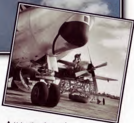
▲ Using the wings and other major components of the B-29, Boeing was able to develop a large transport which was to become the basis of the USAF tanker fleet.
